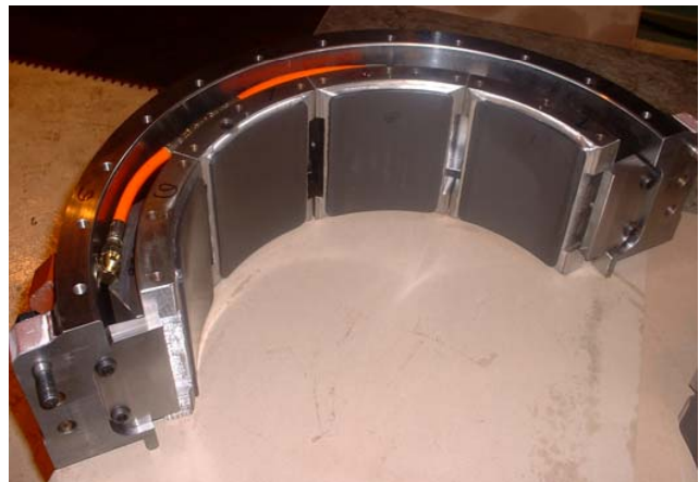
Fig.12 Half assembly PTFE faced journal pads
