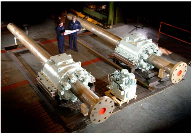
Fig. 11 The TSL bearings complete with shafts and hydraulic actuator positioning unit
