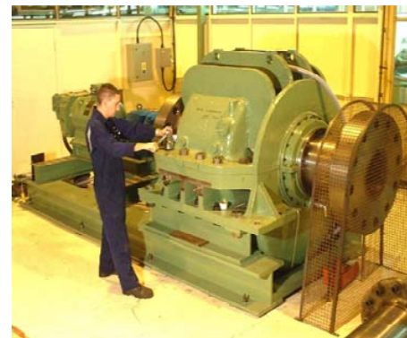
Fig. 2 Submarine thrust block test rig
