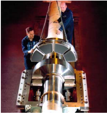
Fig. 10 The TSL thrust bearing with PTFE-faced thrust pads
