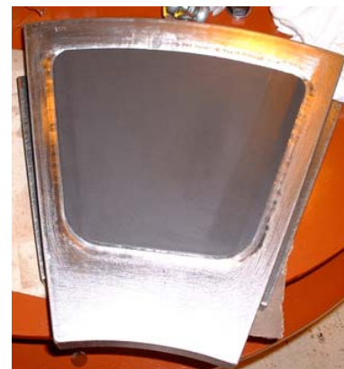
Fig.3 The PTFE faced thrust pad used in test rig
