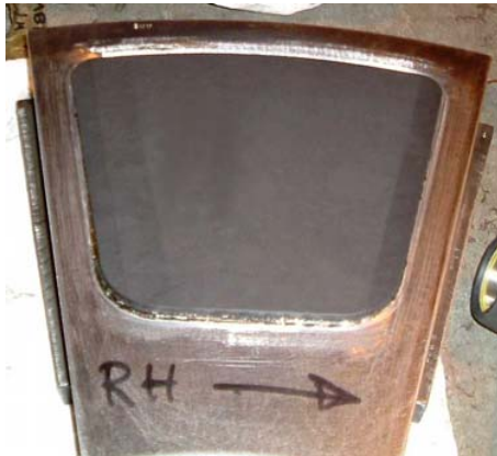
Fig. 4 A PTFE thrust pad after two months testing at 9.6MPa (1392 lbf/in 2 )
